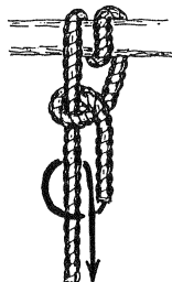
Figure 4. Next, make a half hitch around the standing part of the rope. Then make another half hitch.
