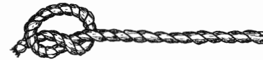
Figure 34. The fisherman's knot is used to join two ropes together by tying two overhand knots. Tie one overhand knot on the end of one rope.
