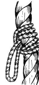
Figure 49. The Prusik can be used on a heavy rope to form a foot- or hand-hold.
