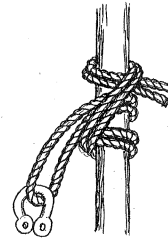
Figure 11. Double the rope and tie the knot to form a loop to attach light tackle.
