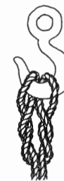
Figure 30. Hook the loops over a hook or spar. A load can be put on both ends or just one end and the knot will hold.
