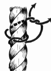
Figure 79. Wrap the whipping cord around the back of the rope and tie another overhand knot.
