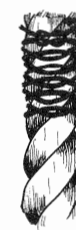
Figure 80. Repeat tying overhand knots, front and back, until the whipping is \frac{1}{4} " to \frac{3}{8} " long. Then tie a square knot to finish the whipping.
