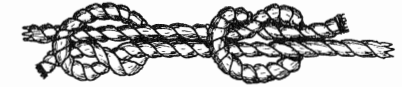
Figure 35. Complete the knot by pulling the second rope through the first overhand knot. Then tie another overhand knot around the first rope.
