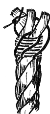
Figure 83. Loop the bight over its strand and tighten it by pulling on end (A). Then finish by tying a square knot, pulling it tight between the strands of the rope.
