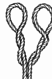
Figure 29. Make at least two twists of each loop, turning the right loop clockwise, and the left loop counterclockwise.
