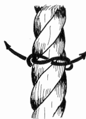
Figure 78. Use waxed flax cord and tie an overhand knot about \frac{3}{4} " from the end of the rope.
