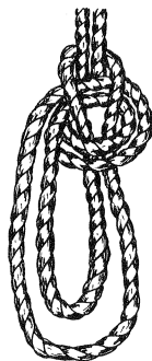
Figure 39. The completed knot has two loops that can be adjusted in size before pulling it up tight.
