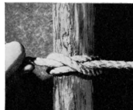
Push loops together and tighten by pulling both ends to complete the knot.
