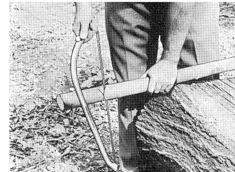
Cut straight down to the depth of side cuts and make a second vertical cut to one side of the first cut.
