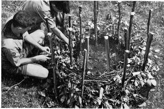
Start a coracle by placing twenty 2-foot stakes in two concentric circles, the inner circle 5 feet in diameter.
