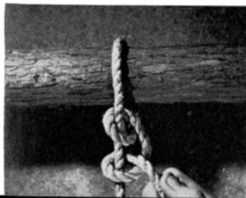
Make second half hitch in front of the first by repeating the process.
